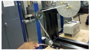
7. Then, run the fiberglass core through the resistance measurement box and the front cylinders.
