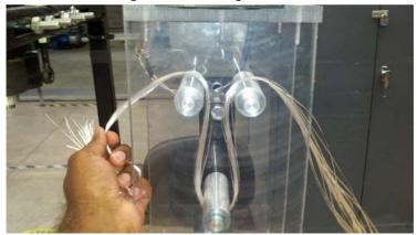
8. Turn on switch "#1". The front cylinders will start rotating. Insert the tip of the fiberglass core midway between the rotating cylinders.
