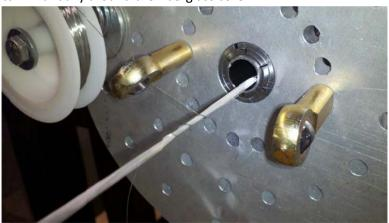
12. Now hold the free end of the wire, and rotate the metal disc by hand forward a few revolutions. This is to make sure that the wire is winding correctly around the fiberglass core. At this stage, also check the tension in the wire. If the tension is too low, adjust the bolt behind the metal disc and tighten. Then rotate the metal disc once again and recheck the tension in the wire.
