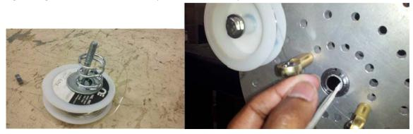
11. Now pass the wire from the spool through the 'eye' mounted on the metal disc and wind a few turn manually around the fiberglass core.
