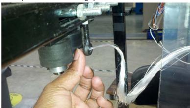
9. Once the fiberglass core is pulled in by the cylinders make sure that it is approximately centered. Turn off switch '#1".
