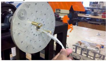
6. Run the fiberglass core through the middle cylinders.
