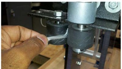
10. Now mount the wire spool on the metal disc and hand-tighten the bolt. The amount of tightening should be such that the spool does not freely rotate.
