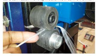
4. Insert the fiberglass core through the hollow tube driven by the motor.
